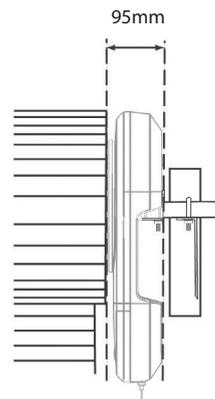
Minimum distance from edge of curtain to edge of door bracket 45mm
